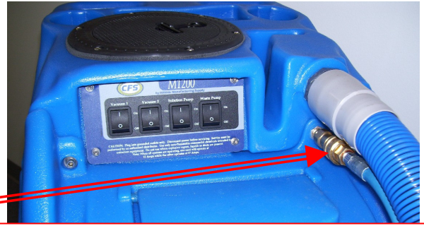
Connect the male end of the HP Solution Hose Assembly to the female solution outlet fitting on the machine. Connect the female end to the cleaning tool.
