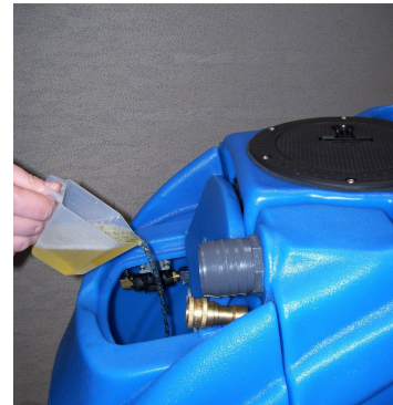
Add appropriate amount of chemical to the hot water in the solution tank
