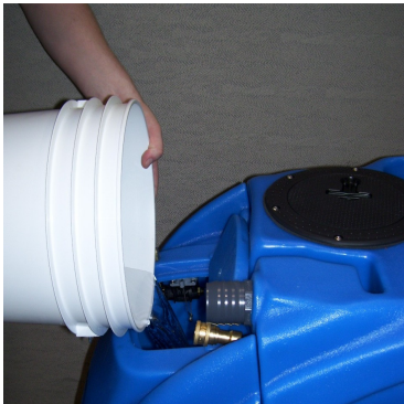
Pour the appropriate amount of hot water into the solution tank
