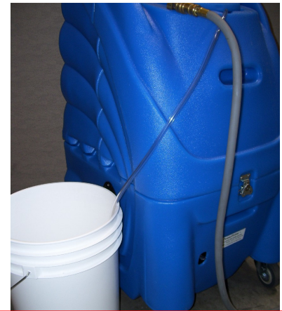
Place Chemical Feed Hose into Rinse Solution
