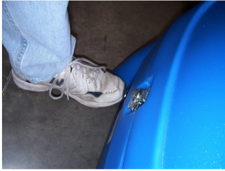
Push & hold the pump priming valve
