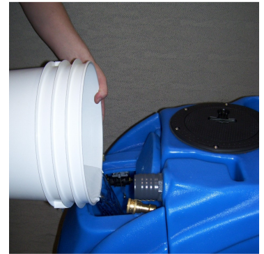
Pour 2 or 3 gallons of clean water into Solution Tank
