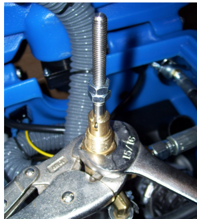
Loosen & remove Stem Retainer from regulator body
