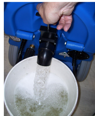
Drain water from Recovery Tank
